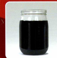
Black iron oxide sludge deposited in a container...
